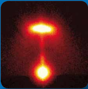
GISAXS pattern of an unaltered multilayer mirror
