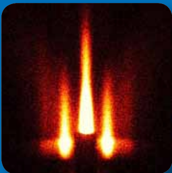
GISAXS pattern of a nanostructured surface
